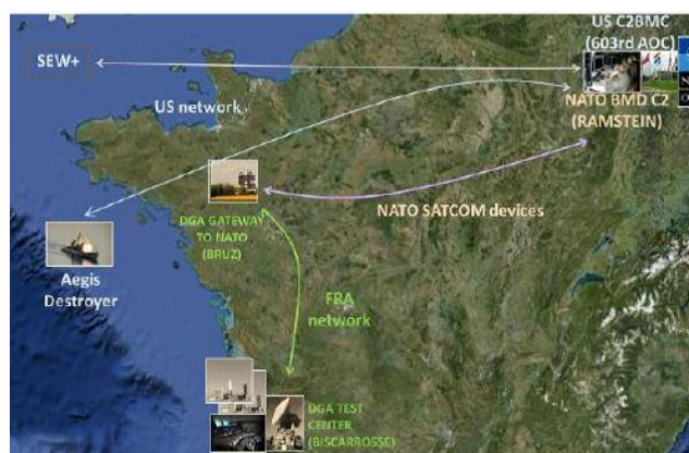
Figure 5: The architecture of the missile defense during the live firing, from bottom to top. The Franco-Italian crew operated 2 SAMP/T sections and intercepted a ballistic target, representative of a SCUD type short range missile. The designation of the SAMP/T was done by a local radar situated in Biscarrosse via a L16 datalink. The chain of command consisted of a French C2 center at Bruz which assured the interface with the command center in Ramstein, regrouping the NATO BMDOC with the ACCS system and the US C2BMC command center, linked with an American Aegis destroyer.
