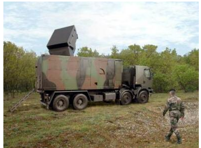
Figure 8.1: The ARABEL fire control radar module « The Eye», with the link of the command missile.
