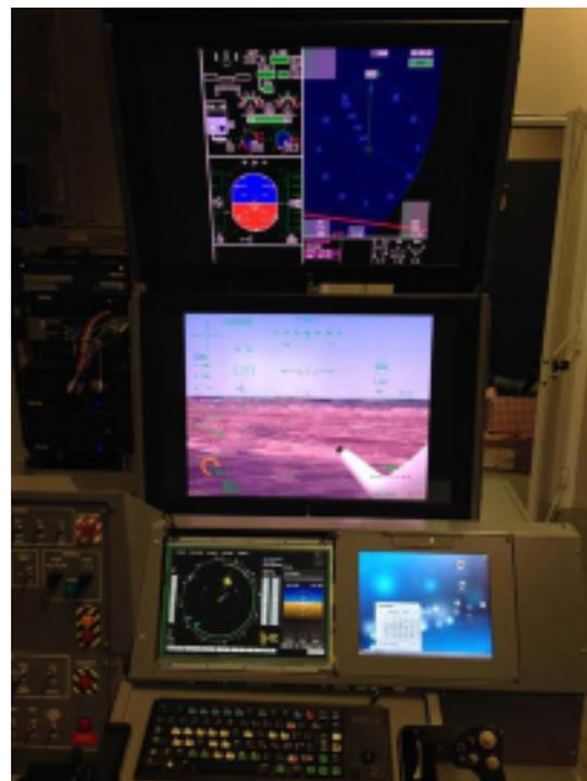
Inside the GCS (Ground Control Station) for the MIDCAS UAV demonstrator. (EDA)
