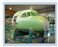
Aerostructures assembly and industrial capabilities for component manufacturing such as Sheet Metal, Surface Treatment, Manual and semi-automatic Painting Cabin and Electrical Harnesses Shop
