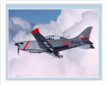
Design & Production of PZL-130 Orlik TC II 750HP (first flight 2003), a fully aerobatic, turboprop, twoseat military trainer used by the Polish Air Force (PAF)
