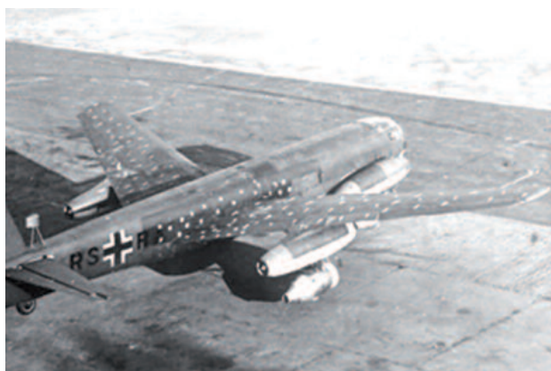
Figure 2. The book contains considerable material on aircraft swept wing with the definite intention of improving the critical Mach Number condition. One of the most interesting is the forward-swept wing Junker 287: see above a picture of the Ju 287 prototype.
