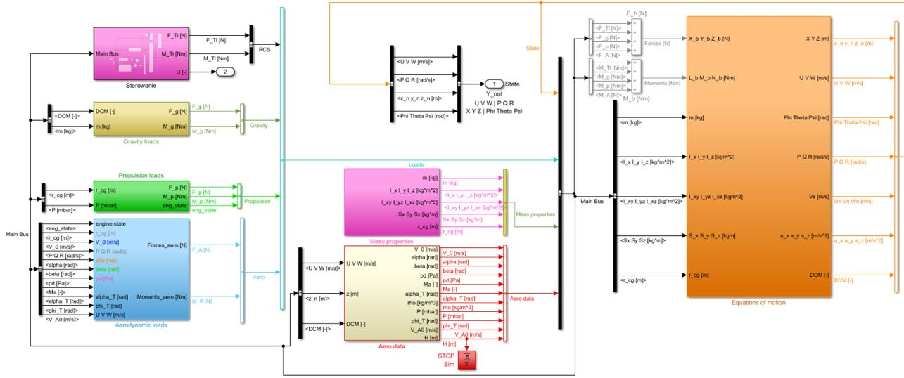
Figure 2 – Missile's mathematical model schematic
