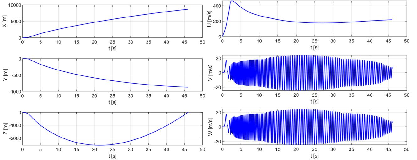
Figure 4 – Missile's trajectory components in North-East-Down frame (left) and linear velocity components in Body frame (right)
