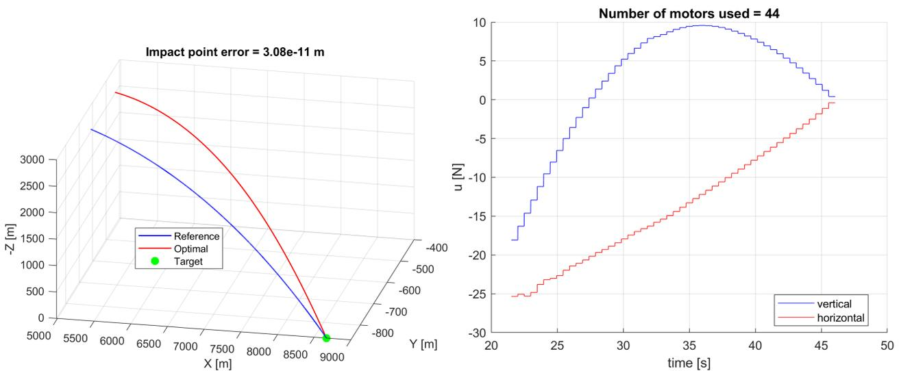
Figure 5 – Missile’s trajectory after optimization in North-East-Down frame (left) and resulting optimal values of the control parameter (right) for case 1
