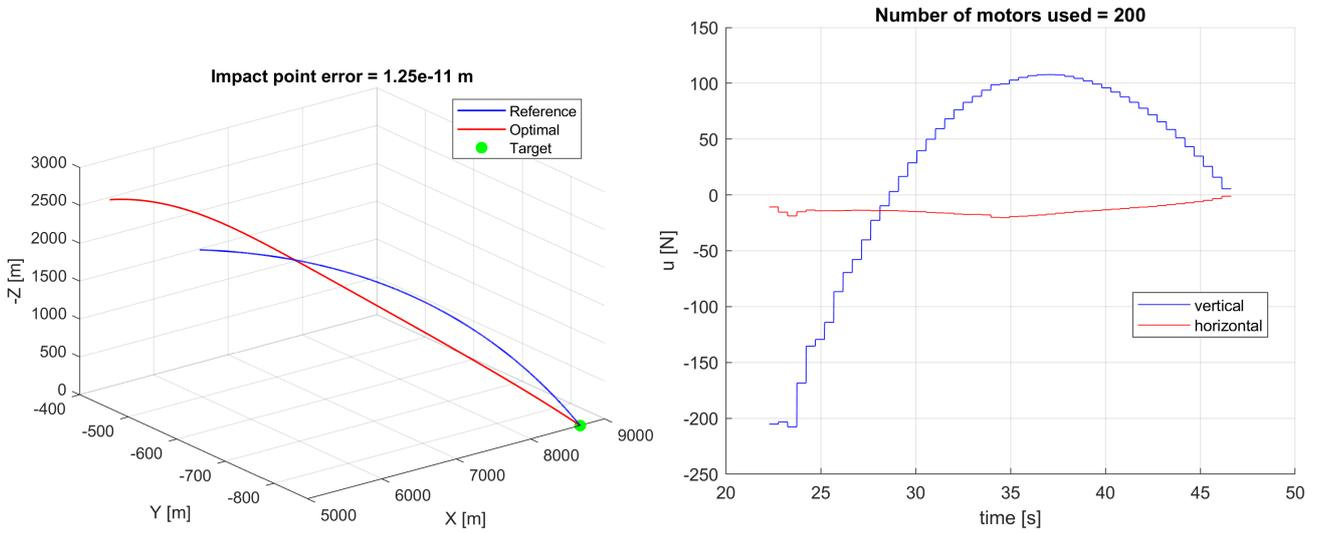
Figure 7 – Missile’s trajectory after optimization in North-East-Down frame (left) and resulting optimal values of the control parameter (right) for case 3
