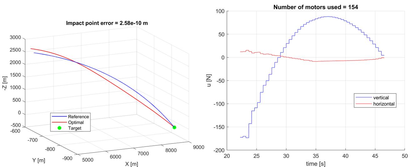
Figure 6 – Missile’s trajectory after optimization in North-East-Down frame (left) and resulting optimal values of the control parameter (right) for case 2
