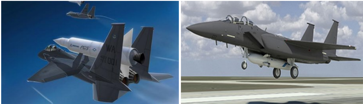
Figure 1 - Evolution in the configuration of Boeing's air-launch-to-orbit systems, on the left: F-15 Global Strike Eagle with a rocket on top of its fuselage, on the right: F-15E ALASA with a rocket underneath the fuselage.
