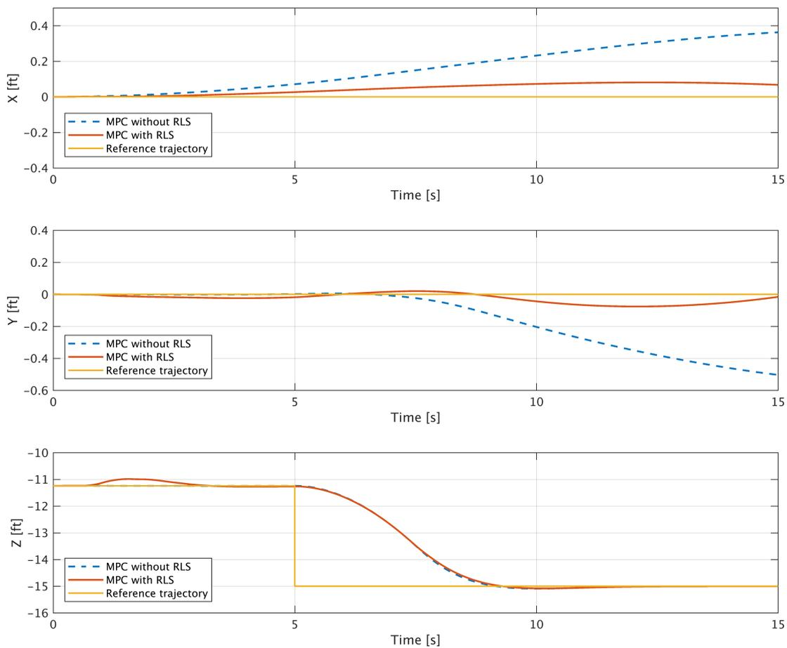
Figure 3 – Case 1, flight level change using MPC with and without RLS model parameter estimation
