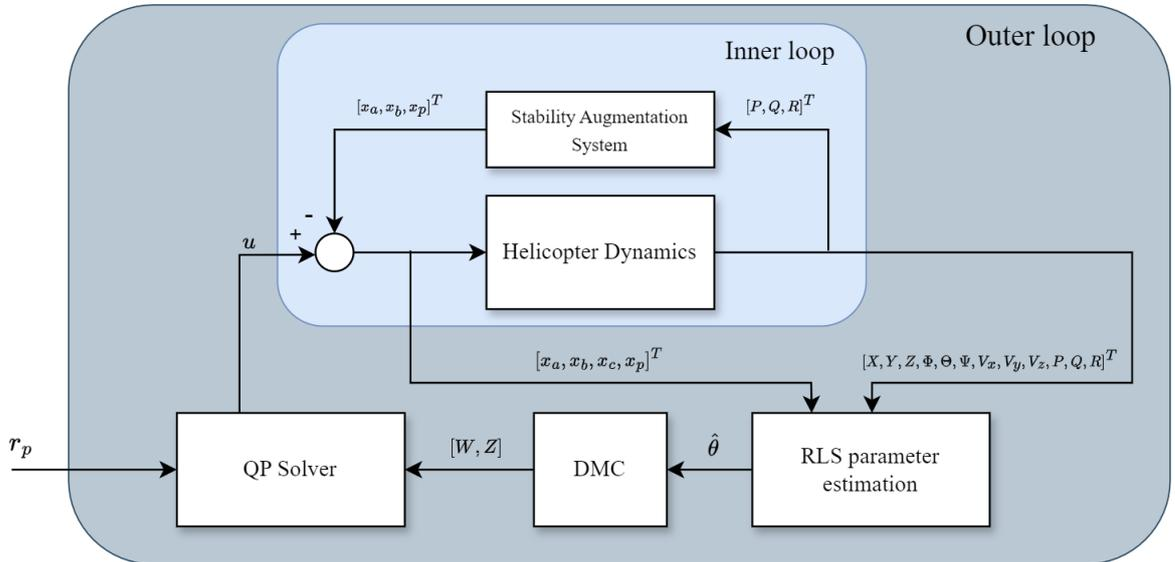
Figure 2 – Automatic Flight Control System scheme
