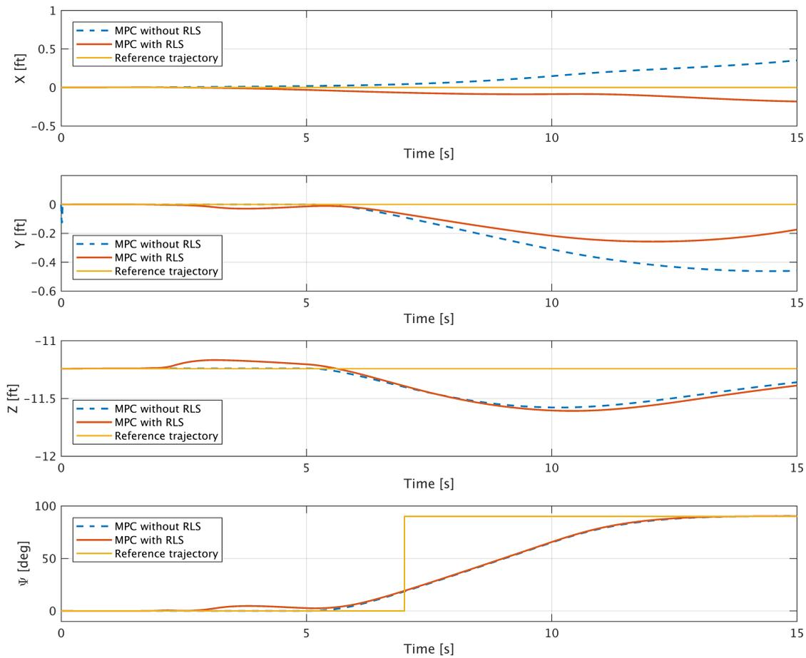
Figure 5 – Case 3, yaw angle change increase using MPC with and without RLS model parameter estimation
