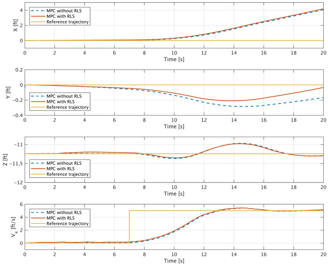
Figure 4 – Case 2, forward flight velocity increase using MPC with and without RLS model parameter estimation
