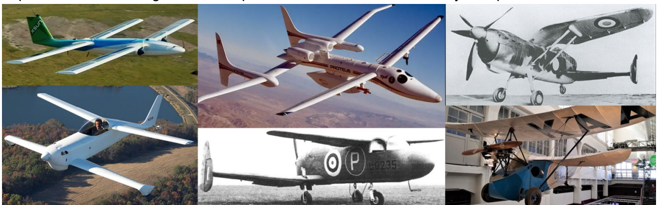
Figure 1 - Tandem wings. Left column: SolarXOne [5], Rutan Quickie [6]; middle column: Scaled Composites Proteus [8], M39B Libellula [9]; right column: Arsenal-Delanne 10 [7], Pou de Ciel [8].
