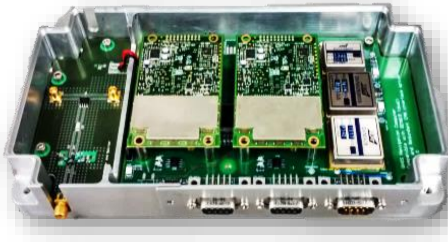
Figure 2 – ESEO GNSS Navigation subsystem.
