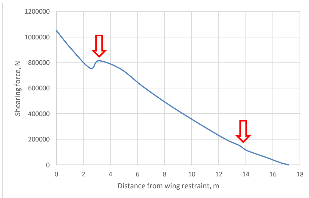
Figure 5 – Shearing forces working on a wing of Boeing 737-800.
