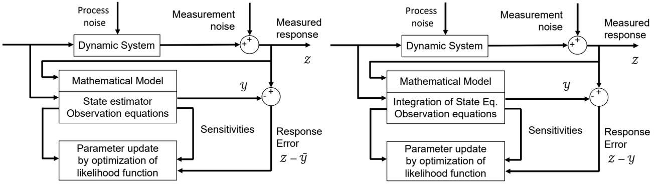
Figure 2 – a) Filter-Error Method. b) Output-Error Method Process [4].
