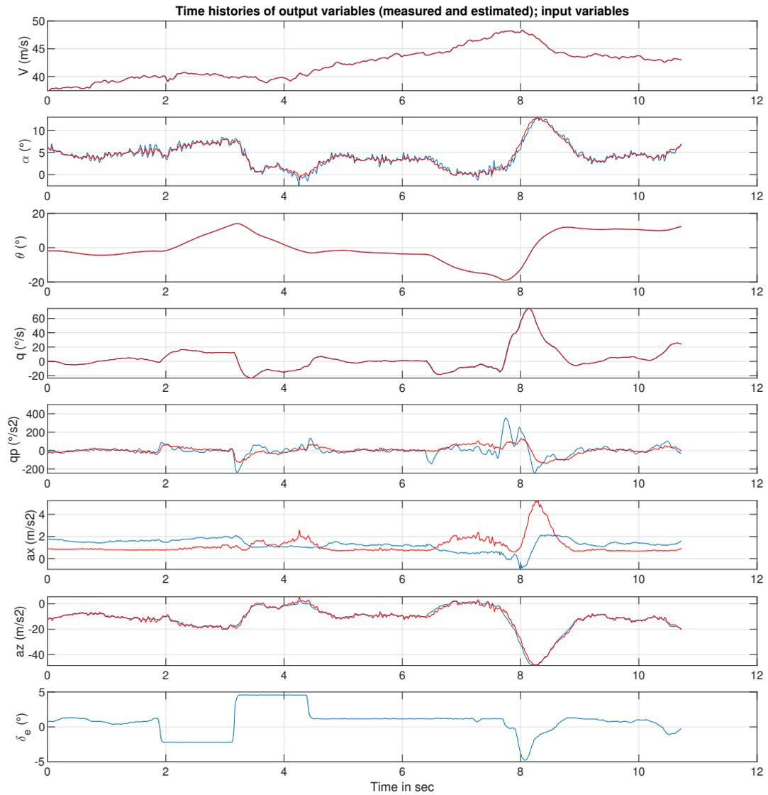
Figure 4 – Filter-Error Method Results
