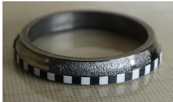
Figure 10 - Faulty bearing inner ring
