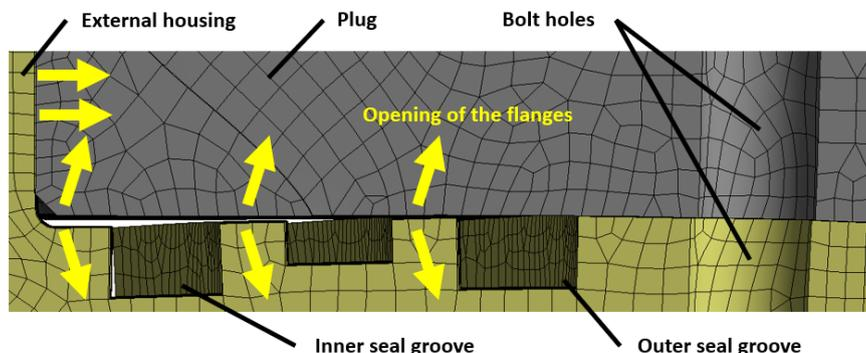
Figure 8 - Seal gap analysis
