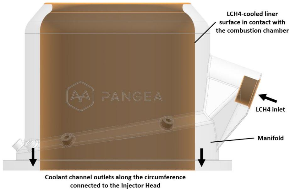
Figure 3 - Cooling of the External Housing
