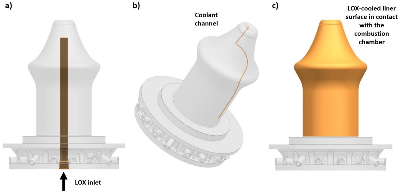
Figure 4 - Cooling of the Plug: a) inlet tubular structure b) spiral coolant channel c) liner surface
