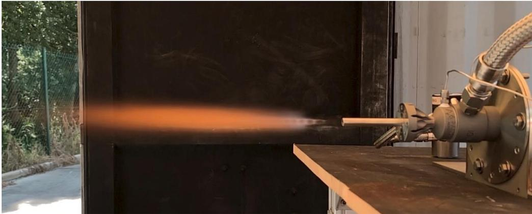
Figure 11 - Igniter hot-fire test
