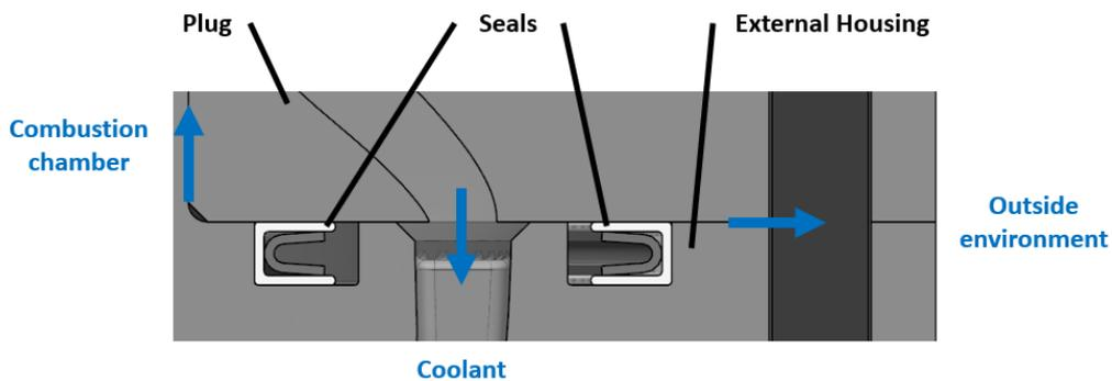
Figure 6 - Seals between Plug and External Housing
