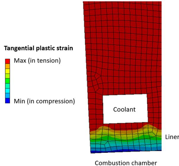
Figure 9 - Tangential plastic strain distribution during hot-firing of the engine
