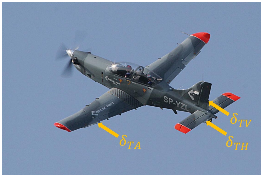
Figure 1 - Trim tabs location on PZL-130 Orlik aircraft.
