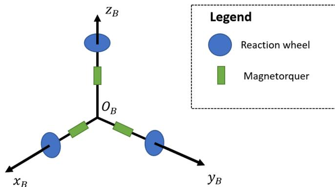
Figure 4: Orthogonal configuration of actuators
