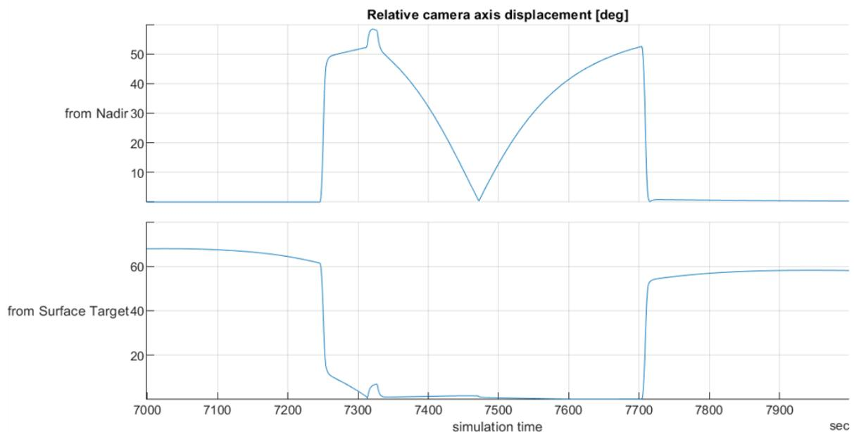
Figure 7: Camera angles in Arm and Acquisition modes in the system-level test
