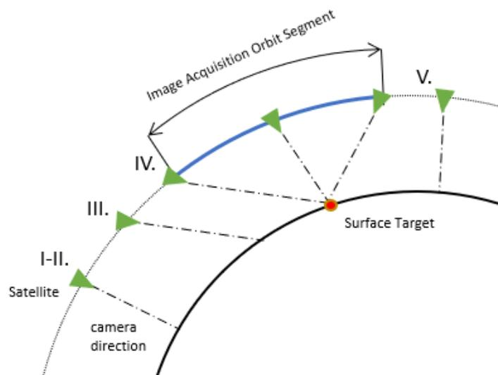
Figure 2: Satellite attitude control during the image acquisition
