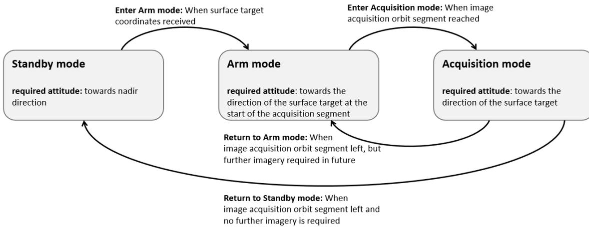
Figure 3: Attitude Control System modes of operation
