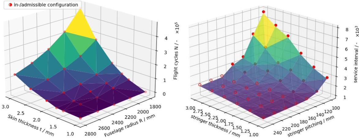
Figure 2: Flight cycle response surface for skin thickness and fuselage radius variation for type II loading (left) and service interval response surface for stringer thickness and stringer spacing variation for type I loading (right)
