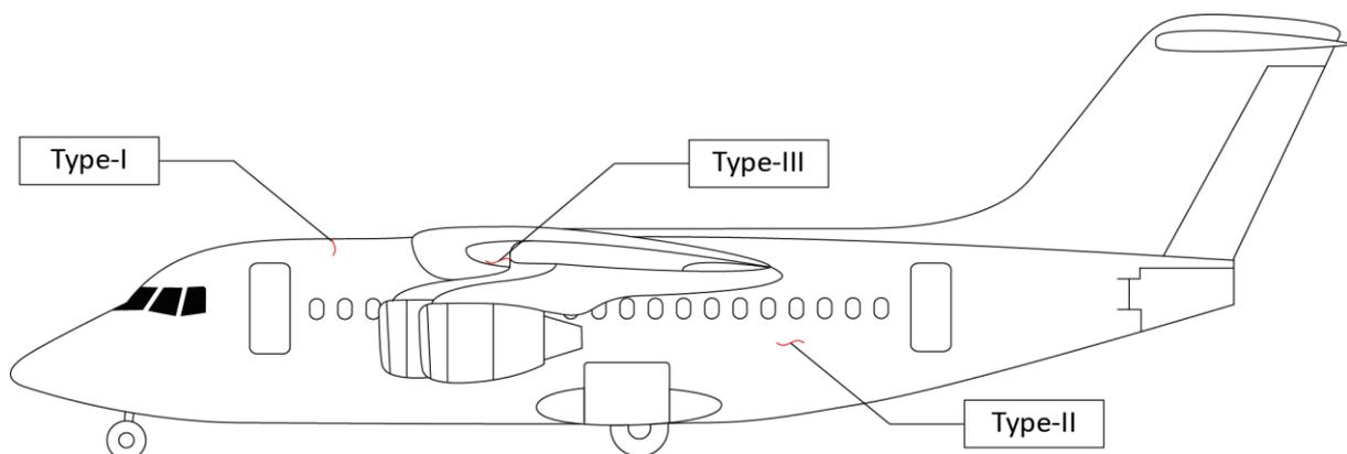
Figure 1: Typical structural elements, crack position and orientation<sup>1</sup>
